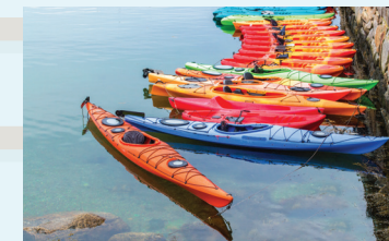
Canoes made from moulded GRP
