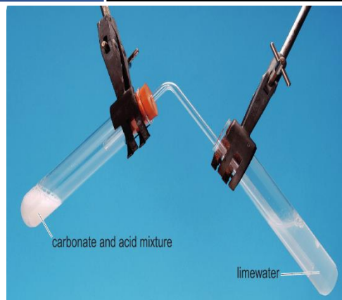
B using limewater to confirm the results of a positive test for carbonate ions
