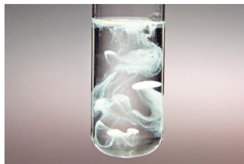
C A white precipitate of barium sulfate forms in a positive test for sulfate ions.
