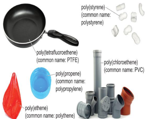
A There are many different polymers and their uses depend on their properties.
