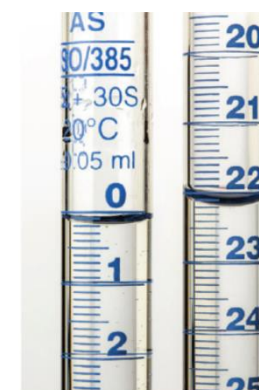
B The initial volume of solution in the burette is 0.20 cm 3 and the final burette reading is 22.20 cm 3 .
