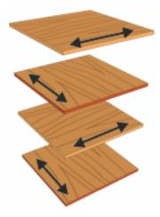
Manufactured boards can be either be made by lamination or compression
